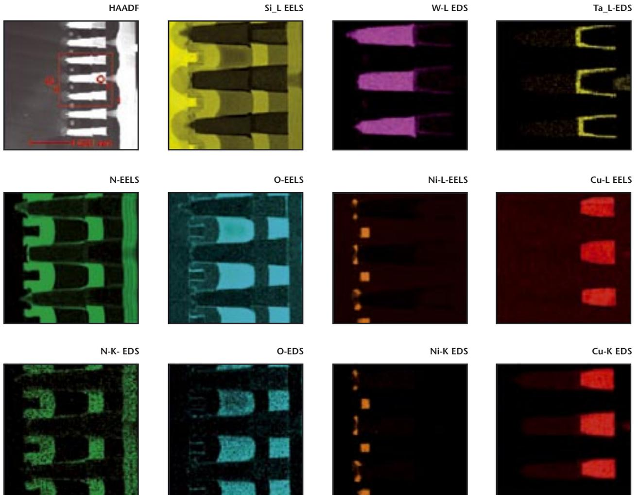
Simultaneous EDS and EELS map on IC device at 300 kV.
