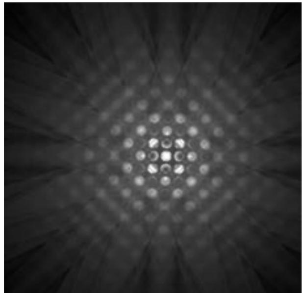
Energy filtered convergent beam diffraction.
