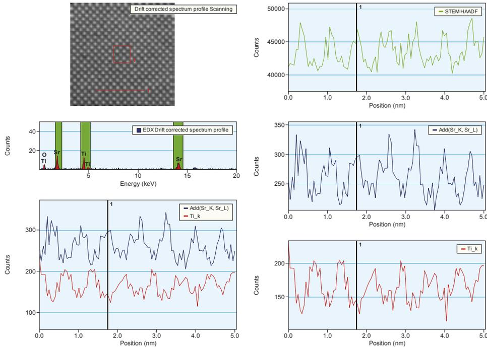
EDS and HAADF signal has been acquired at the same time. Drift correction using cross correlation methods has been used on the marked red square. The red line indicates the profile position in the HAADF image.
