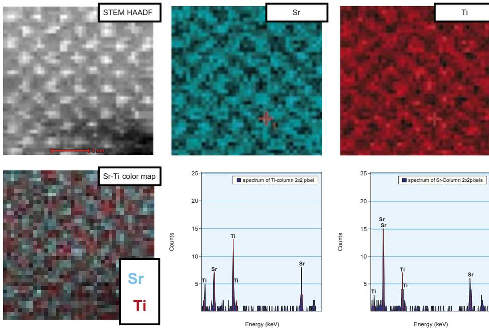
Direct imaging of the Sr and Ti sub-lattice with EDS in SrTiO<sub>3</sub> in <100> direction. EDS and HAADF signal has been acquired at the same time. Drift correction using cross correlation methods has been used on the marked red square. The spectra shown indicate the EDS signal at the Sr and Ti position of the lattice. The color map shows clearly the sub-lattice of Sr and Ti in the unit cell.
