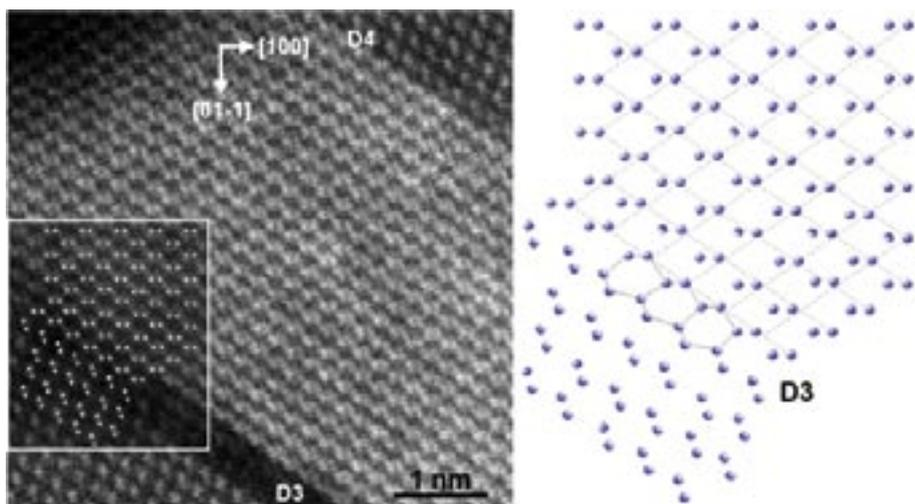
The atomic structure of the defect line D3 as determined from the micrograph is overlaid and separately shown on the right. The defect line D3 does not show the ideal symmetry of a S3 CSL twin boundary.
