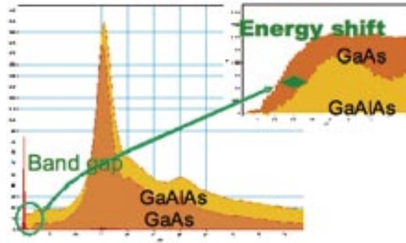
Shift in band gap energy and plasmon loss due to Al-dopant can be measured.
