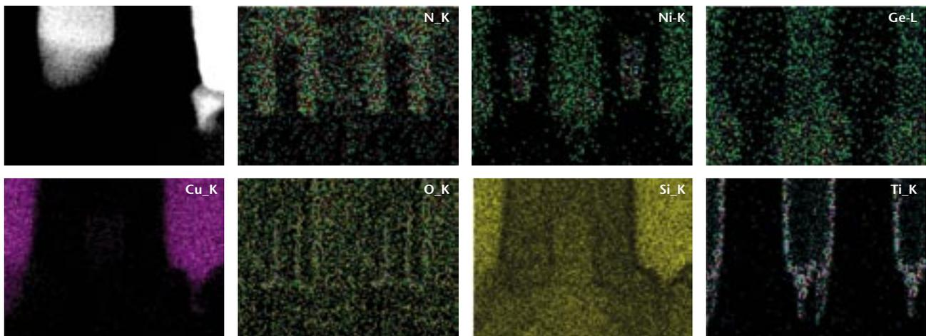
EDS-map with 3 nA probe current 128 x 100 pixel, 0.2 ms per pixel 32 times -> 1½ minutes.
