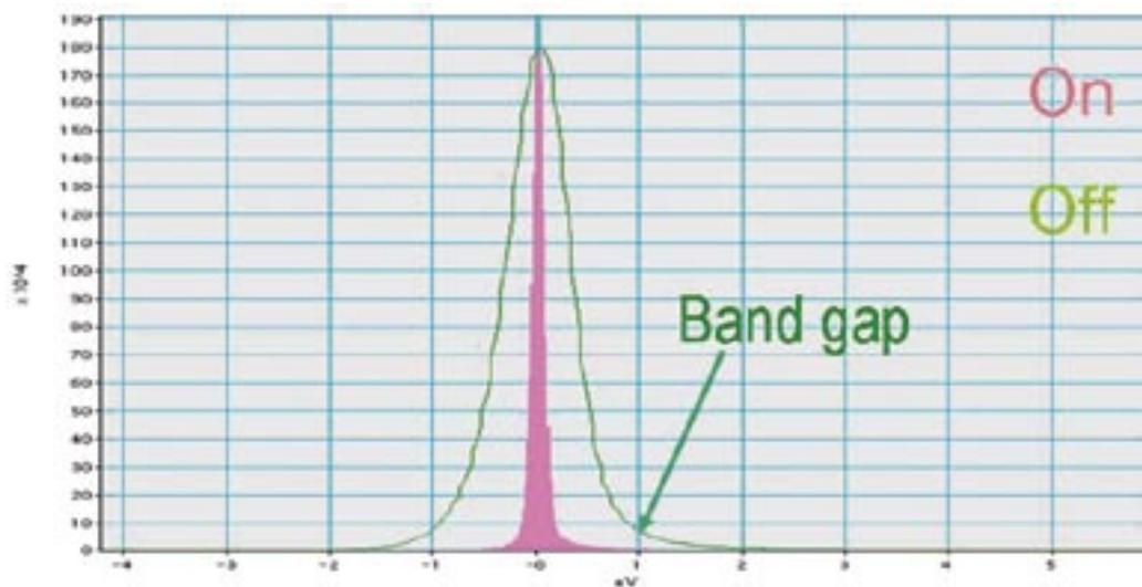
The long tail of the zero-loss reaches into the area of the band gap energy and increases the background in the area. The monochromator reduces the background dramatically in the area of the band-gap energies (1 - 3 eV).
