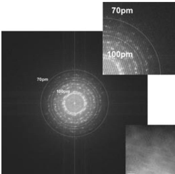
*Mono Off &  $C_s$ -corrector On. Sub-Ångström Young fringe experiment on gold cross grating on a monochromized corrected Titan at 300 kV.*
