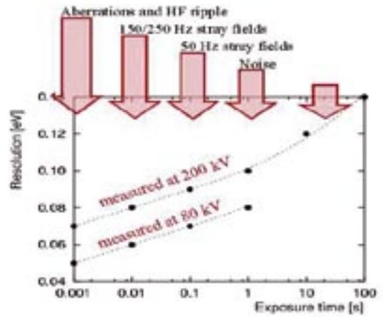
Ultra stable Wien-filter type monochromator with energy resolution  $< 0.2\ \text{eV}$ .
