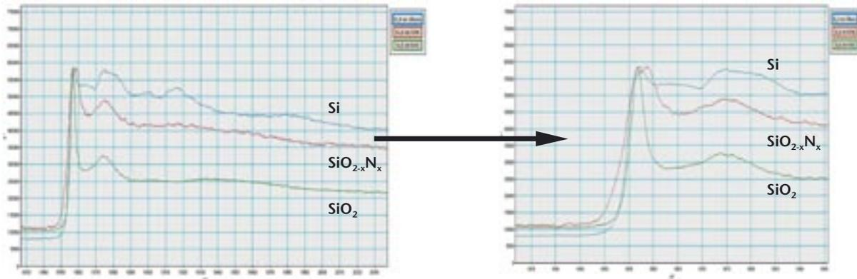
ELNES of silicon-k edge (DE = 1860 eV) in Si, SiO<sub>2</sub> and SiON.
