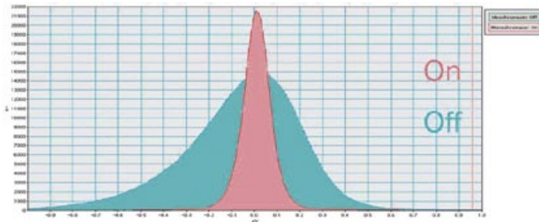
Energy resolution @ 300 kV using FEI monochromator with Gatan Tridiem 866.
