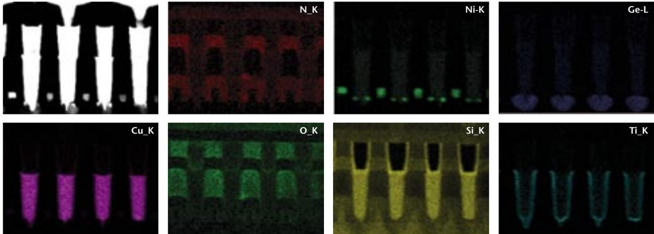
EDS map with 3 nA probe current 256 x 200 pixel, 0.2 ms per pixel 64 times -> 11 minutes.
