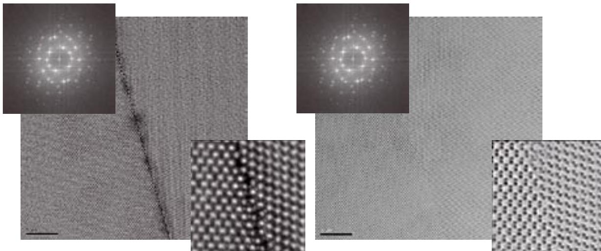
Comparison of HR-TEMs with and without  $C_s$ -correction on the same  $Si\langle 110 \rangle$  grain boundary at 300 kV. Images: B. Freitag (FEI). Sample courtesy of: J. Thibault, Marseille.
