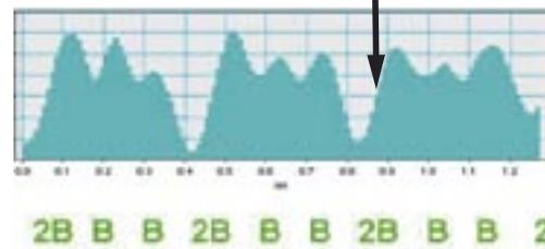
Direct imaging of boron atoms in the [001] zone axis of  $LaB_6$ . Boron distance of  $\sim 120$  pm can be resolved. A contrast difference between differently occupied boron columns (single and double in unit cell) is noticeable.
