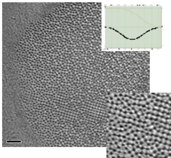
Comparison of HR-TEM images on the same area of  $Nb_7W_{10}O_{47.5}$  at 300 kV. The determination of the atomic position in the corrected images is easier, because every atomic distance is transferred with the same contrast (see the contrast transfer function).
