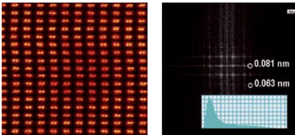
Ge 112: acquisition time 20 s, frame size 512 × 512 pixels; FFT shows up to 0.63-Å resolution. Histograms confirms that the signal is not clipped (probe semi-angle 25 mrad).
